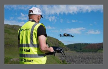
The Falcon 8 gives you full control over your flight planning. Manually fly the Falcon 8 around the object to be inspected, or program your flight path in advance. Save your accomplished flight path and repeat it automatically for exact comparison during a next inspection.
